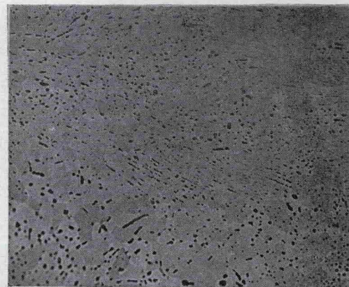
FIG. 9(b). The microstructure of a 90% Sn-bal Bi specimen where pressure at fracture equalled 1.55 \times 10^8 \text{ N/m}^2 . Note the smaller grain size than that shown by Fig. 9 (a) and lack of particle-matrix separation. 500 \times , Unetched.
